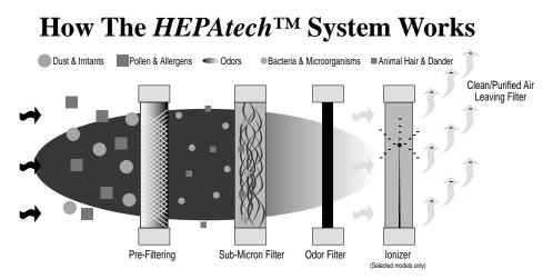
The above is an illustration of how the *HEPAtech<sup>TM</sup>* air purification systems work. Dust and other irritants are pulled into the air purification system and cleaned through the *HEPAtech<sup>TM</sup>* Filter. Clean, purified air is released into the room.
